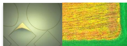
Drilling and cutting green tape (L) and solder mask removal (R).
